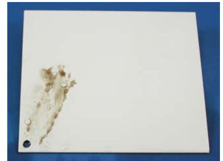
Figure 4: After rinsing, the hydrophilic right side of the panel readily releases soil.
