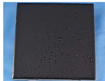
Figure 1: Untreated ceramic tile exhibits hydrophobic nature.
