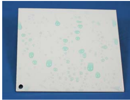
Figure 1: Untreated panel exhibits hydrophobic nature.
