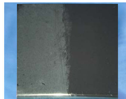
Figure 3: After 10 soiling/rinsing cycles, the right side of the tile is still hydrophilic and is a barrier to soap scum buildup and hard water spotting. The untreated left side allows soap scum buildup and hard water spotting.
