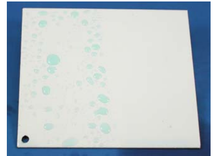
Figure 2: Right half of panel treated with 0.5% Flexipel SR-80 exhibits complete hydrophilization.
