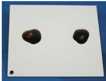
Figure 3: Dirty motor oil is applied to dried panel. Untreated (left) and treated (right).
