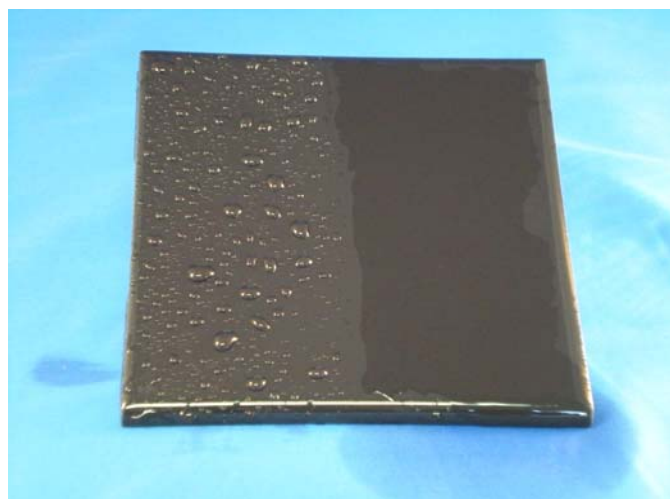
Figure 2: Right half of tile treated with a formulation containing 1.0% Flexipel SR-95HF exhibits hydrophilic barrier properties.
