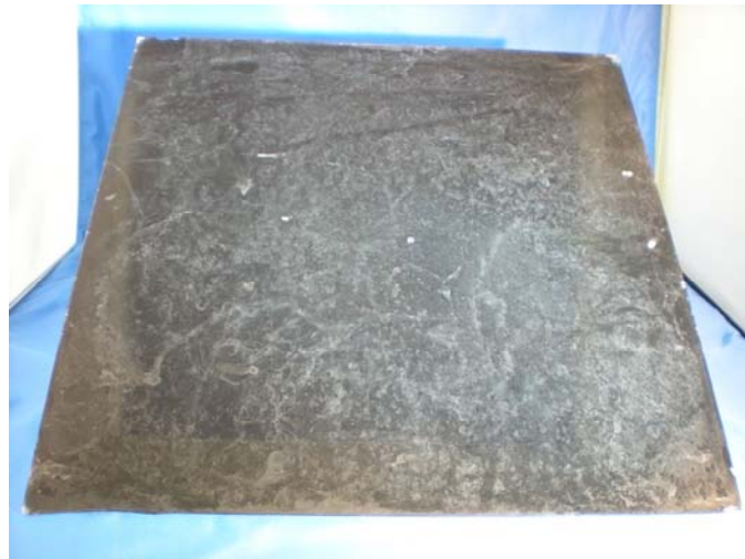
Figure 1: A glass panel is painted black on its underside. The unpainted side is soiled uniformly with a standard soap scum and hard water solution.
