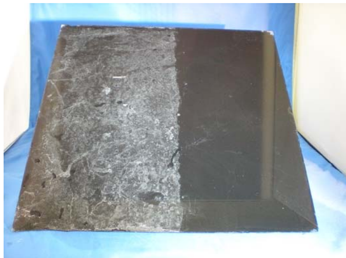
Figure 3: After 10 soiling/rinsing cycles and time to dry, the right half of the glass panel is still hydrophilic and resists soap scum buildup and hard water spotting. The untreated left side allows soap scum buildup and water to spot.
