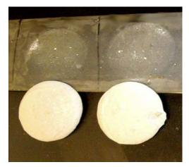
This photo shows concrete cured over a steel test plate. The steel plate was treated with a solution of 1 part Flexipel CR-515 and 9 parts of water. This is the fourth concrete sample to be removed after only the initial application of release agent. Between each sample removal the plate was rinsed with water and allowed to dry, but no additional form release agent was applied.
