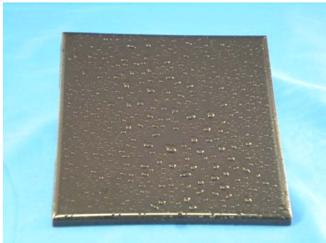
Figure 1: Untreated ceramic tile exhibits hydrophobic nature.
